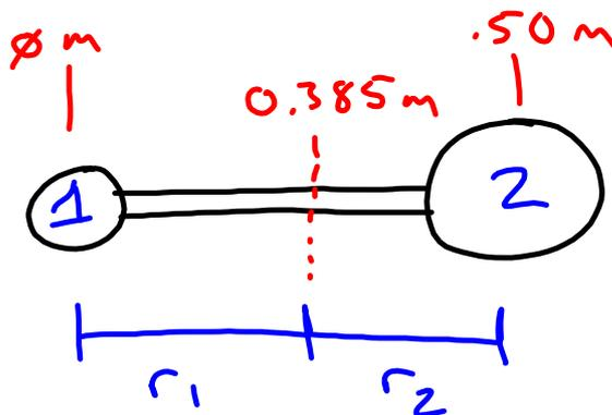
$$v_1 = r_1 \omega = (0.385 \text{ m})(5.236 \text{ rad/s}) = 2.014 \text{ m/s}$$
